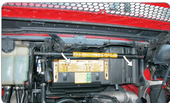
**EN** Remove the protecting device
