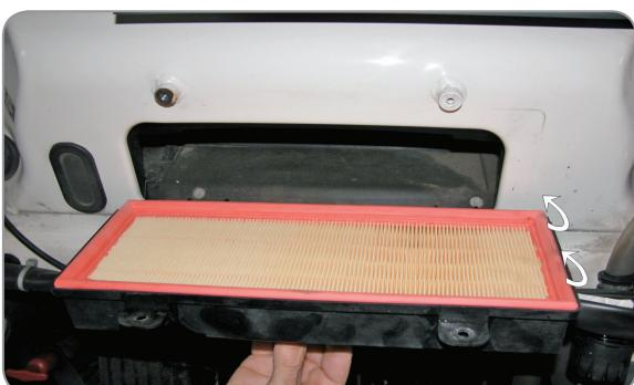
EN Take out the filter with its frame, remove the old filter from the frame and put in the new one
