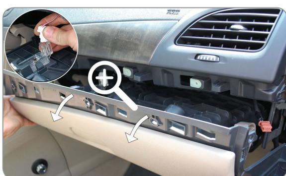
EN Disconnect the electric circuit, remove the glove compartment
