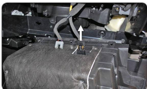
**EN** Disconnect the electric circuit
