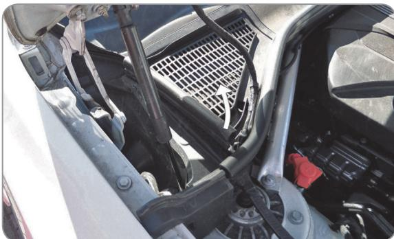
EN Remove the rubber seal
