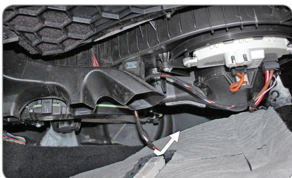
EN Disconnect the electric circuit
