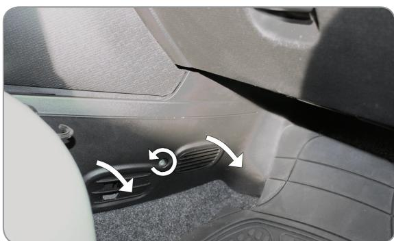
**EN** Loosen the screw and remove the upholstery panel
