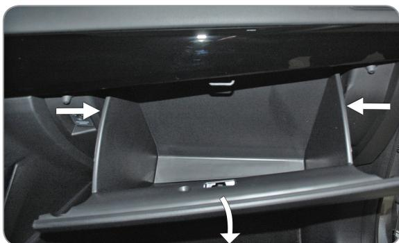
**EN** Remove the glove compartment
