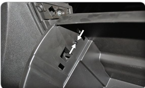
EN Remove the protecting device
