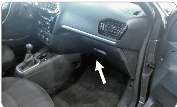
**(EN)** The filter is located under the glove compartment
