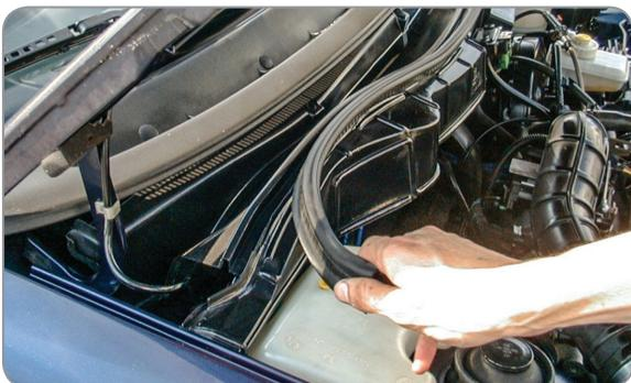
**EN** Remove the rubber seal
