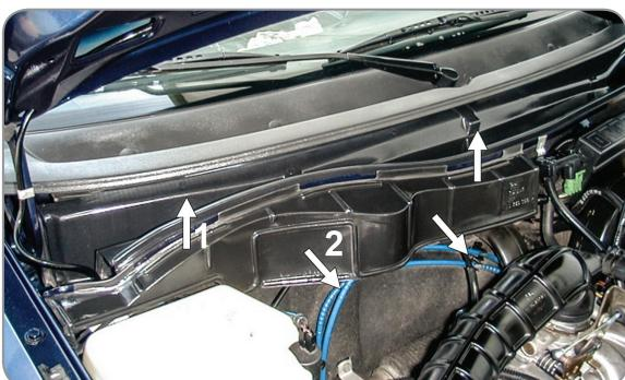
**EN** Remove the electric circuit housing
