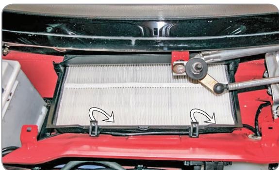
EN Open the locks of the pollen filter. Gently remove the old filter, put in the new one and carry out the opposite to all the previously mentioned operations in the reversed order
