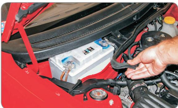
**(EN)** Remove the rubber seal
