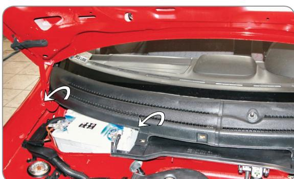
**(EN)** Remove the first section of the screen
