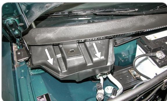
EN Remove the filter housing
