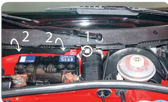
(EN) Remove the protecting device, remove the filter housing
