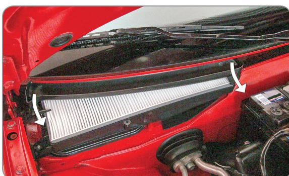
(EN) Remove the protecting device
