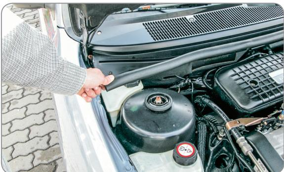
EN Remove the rubber seal
