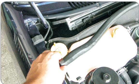
**(EN)** Remove the rubber seal
