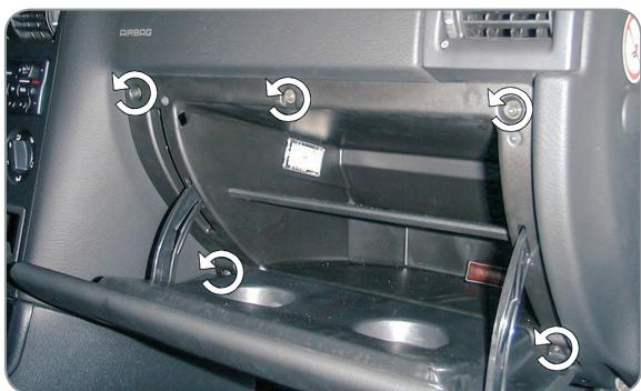
**EN** Loosen the screws and remove the glove compartment
