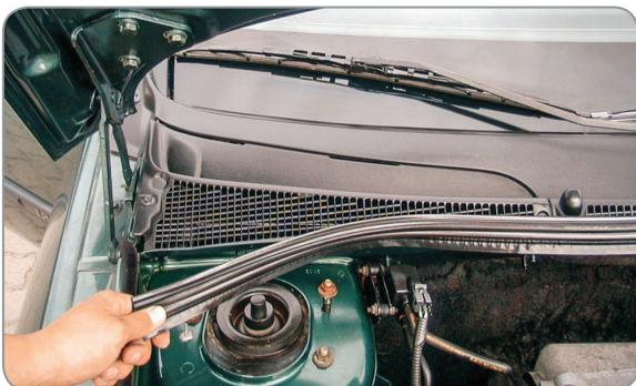
**EN** Remove the rubber seal
