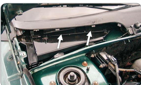
**EN** Remove the cover located above the filter
