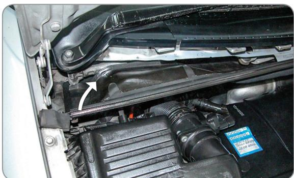
(EN) Remove the rubber seal
