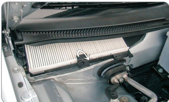
EN Remove the filter lock
