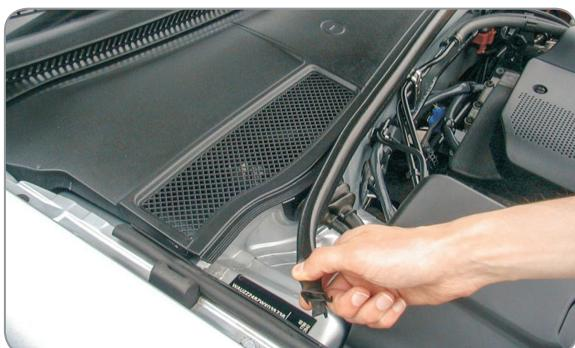
EN Remove the rubber seal
