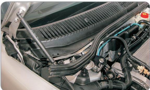
**EN** Remove the rubber seal
