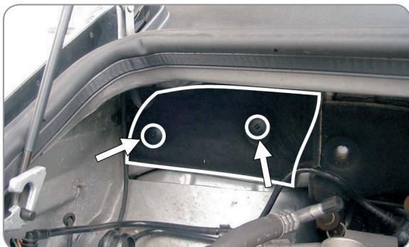
**(EN)** Loosen the screws on the filter housing
