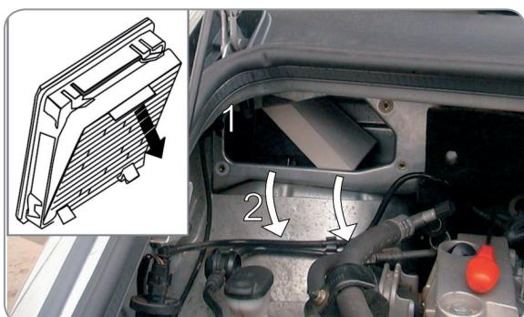
**(EN)** Take the filter out together with the frame. Gently remove the old filter, put in the new one
