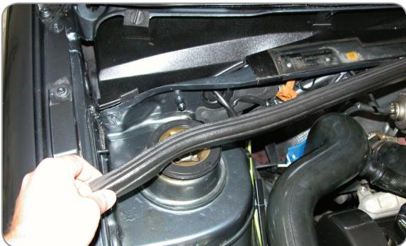
(EN) Remove the rubber seal
