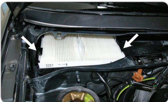
(EN) Unlatch the filter from its socket
