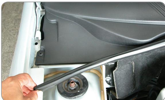
**EN** Remove the rubber seal
