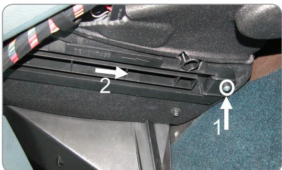
**(EN)** Loosen the screws and remove the cover of the filter
