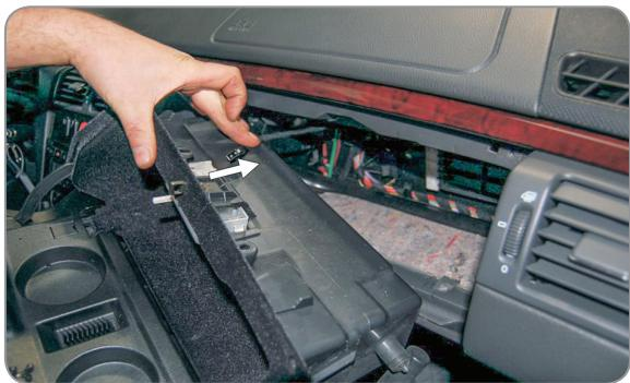
**(EN)** Disconnect the electric circuit
