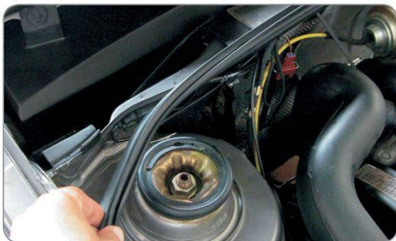
**(EN)** Remove the rubber seal
