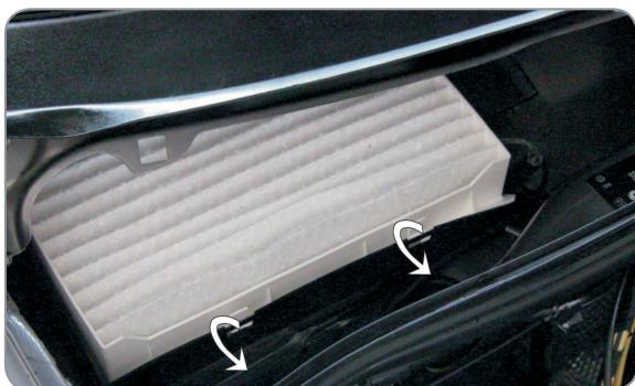
**(EN)** Unlatch the filter from its socket
