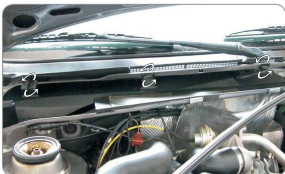
**(EN)** Turn the locking elements of the filter screen 45 degrees to the left
