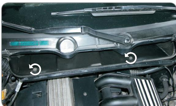
**(EN)** Loosen the screws that hold the cover of the filter chamber
