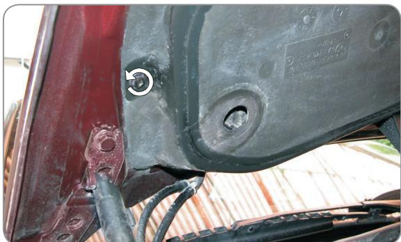
**EN** Loosen the screw on the filter housing
