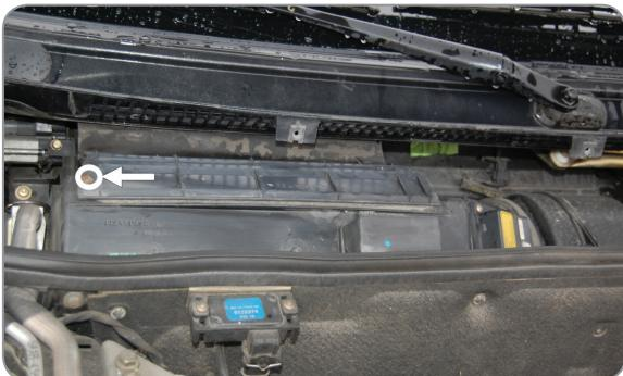
**EN** Loosen the screw on the filter housing, remove the filter housing
