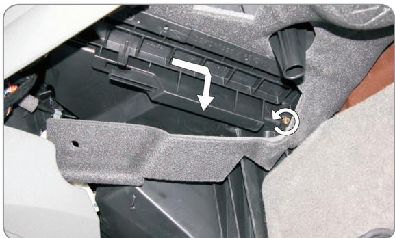
**(EN)** Loosen the screw. Move the filter cover to the right
