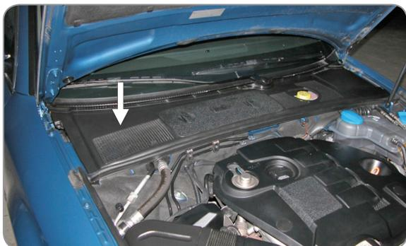
Pollen filter is located behind the engine chamber. Remove the screen under the windshield
