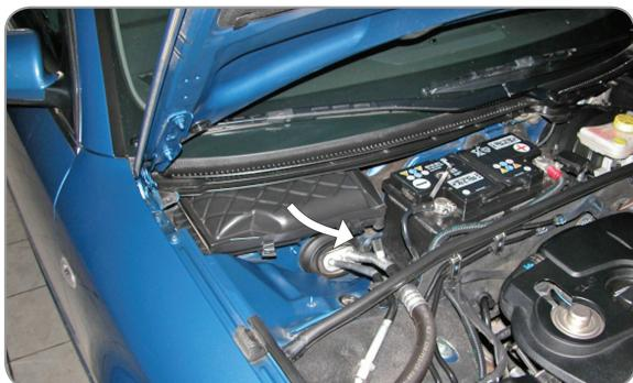
Detach the cover of the filter chamber
