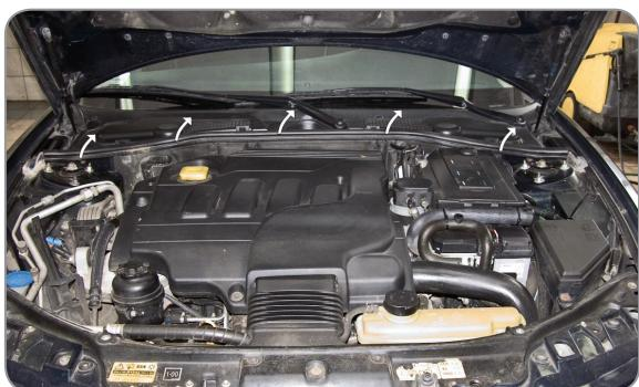
EN Remove the rubber seal
