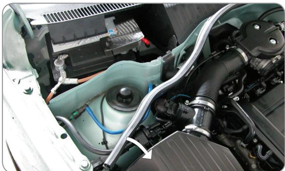
(EN) Remove the rubber seal
