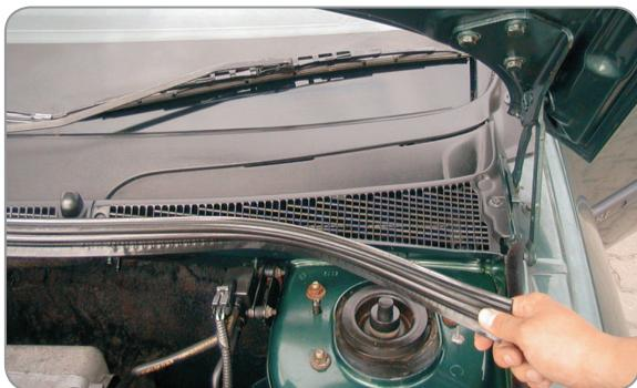
**(EN)** Remove the rubber seal
