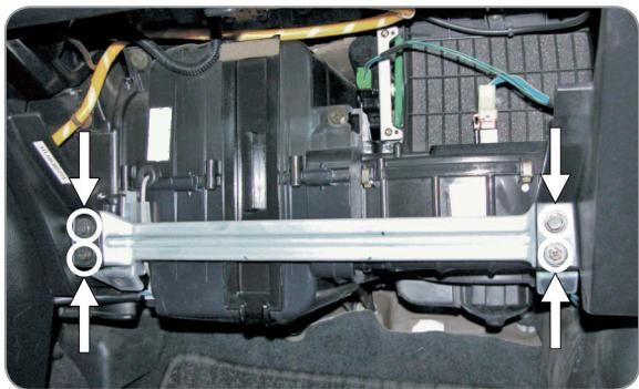
**(EN)** Remove the protecting device
