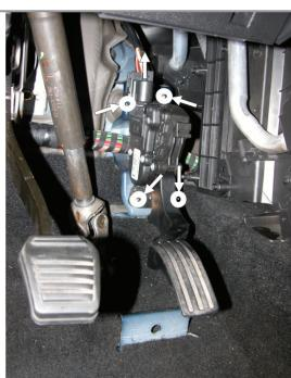
**EN** Disconnect the electric circuit. Unscrew the screws fastening the element shown on the picture
