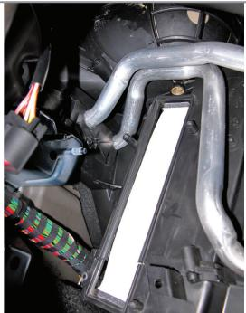
**EN** Gently remove the old filter, put in the new one and carry out the opposite to all the previously mentioned operations in the reversed order
