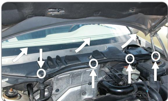
**EN** Loosen the screws of the screen under the windshield. Remove the screen segment
