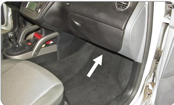
EN Pollen filter is located under the cover of the glove locker
