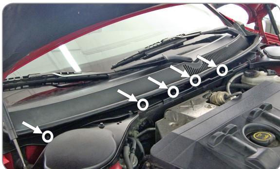
(EN) Loosen the screws, which hold the screen under the windshield
