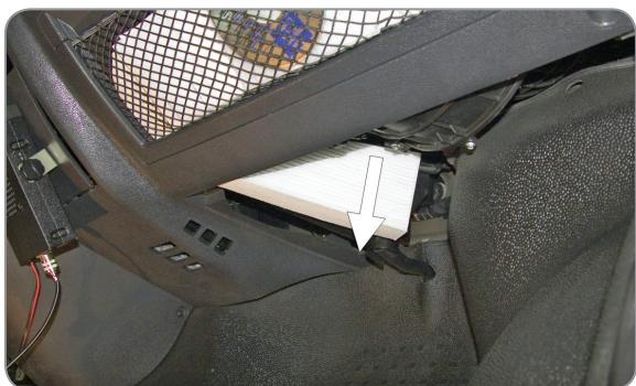
(EN) Change the filter making sure to place the new one firmly in the guide of the filter chamber
