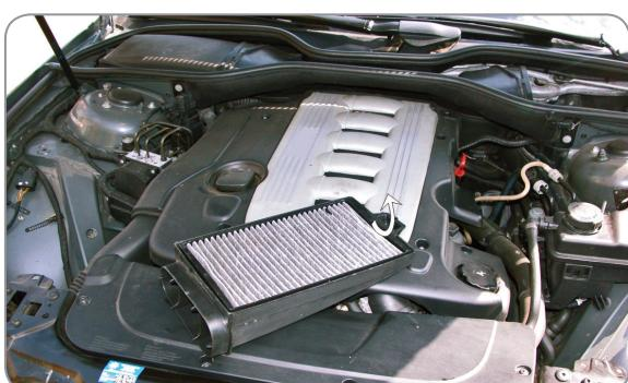
EN Take out the filter together with the frame, remove the old filter from the frame and replace it with the new one, do the same with the other filter
