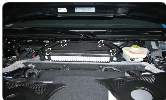
**EN** Loosen the nuts and remove the filter housing
