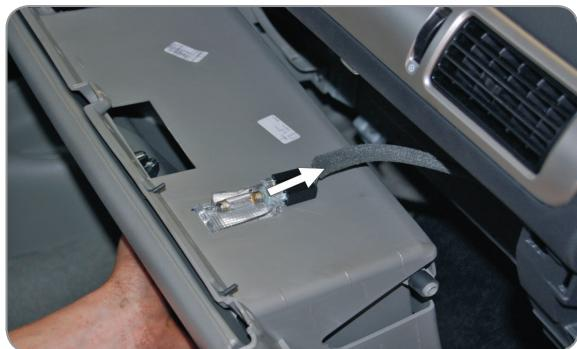
(EN) Disconnect the electric circuit
