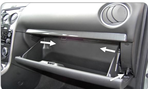
EN Remove the glove compartment
