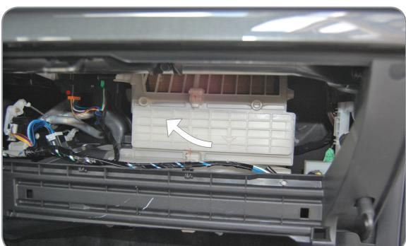
EN Remove the filter housing
