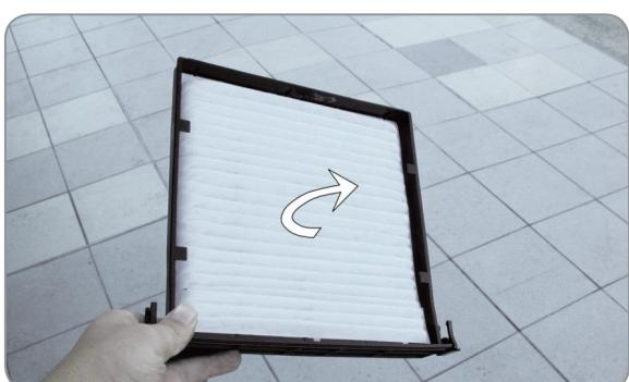
**EN** Remove the filter from the frame, put in the new one and perform the previous actions in the opposite order
