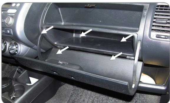
**EN** Remove the glove compartment
