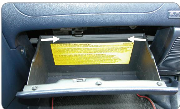
**(EN)** Remove the glove compartment
