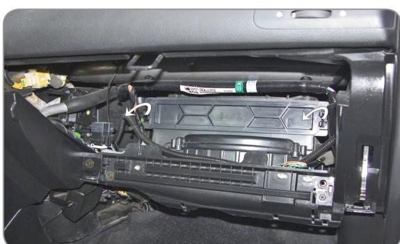
Remove the cover of the filter chamber, remove the old filter from the seat, put the new one in and perform the opposite to all the previous actions in the reverse order
