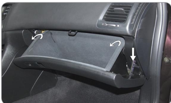
**(EN)** Remove the glove compartment
