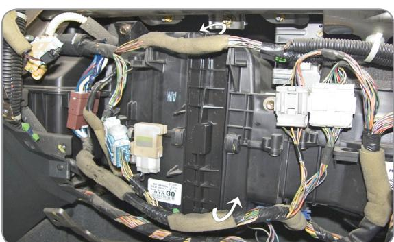
**EN** Remove the filter housing
