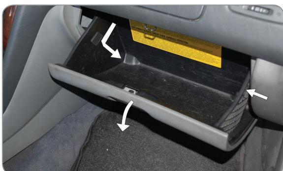
**EN** Open the glove compartment, unclasp the compartment
